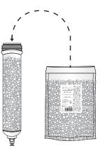
5. Fasten the foam pad and the sieve, then screw the sealing cap back onto the cartridge. Make sure that the seal and the thread are not contaminated with particles of the filter granulate. This could cause the cartridge to leak.
